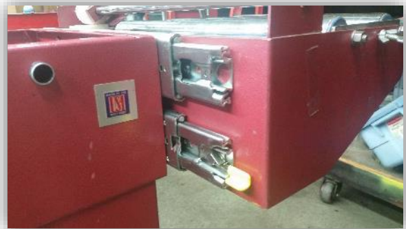
Figure 10: Sliding mechanism attached and slightly extended.
