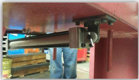
Figure 12: Machine body connection to 10" stroke cylinder.
