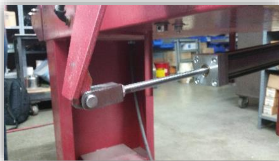
Figure 11: L Bar support connection to 10" stroke cylinder.
